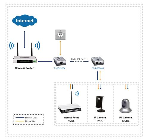
\* TP-LINK's TL-POE200 uses widely adopted PoE technology in the industry and provides more cost-effective PoE solution. It is highly recommended not to pair the PoE200 with other PoE adapters unless under professional guidance.
