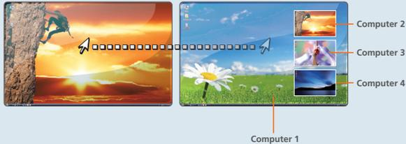
Cursor Shift Function – when you are using two displays, the mouse cursor can move back and forth across the displays, shifting the KVM focus.
