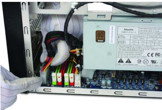
③ Attach the 20-pin ATX and 2x2-pin (or 1x4-pin) power supply plugs to the mainboard.
