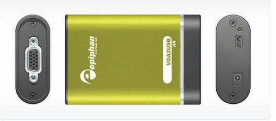
The VGA2USB HR from Epiphan Systems is a frame grabber designed for precise high resolution and high frame rate VGA capture. This device provides the user with a 100% lossless VGA signal grab via features such as the 32MB internal buffer memory, on board lossless frame compression, integrated color space conversion and on board cropping.
